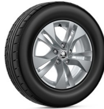
Spitzberg light-alloy wheel 6.0J x 16" ET43 for 215/60 R16 (4x2, 4x4), 225/60 R16 (4x4) 57A 071 496C 8Z8 | silver metallic
