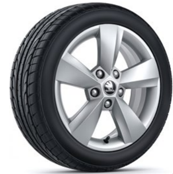
Nanuq light-alloy wheel 6.0J x 16" ET43 for 215/60 R16 (4x2, 4x4), 225/60 R16 (4x4) 57A 071 496A 8Z8 | silver metallic
